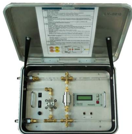
Figure 1-1: Mobile device of horizontal profiles measurement
